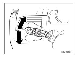
To signal a turn, move the lever all the way up or down. When the turn is finished, the lever will return automatically.
